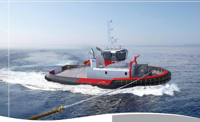
The OST 32 E is the latest addition to the famous OST multipurpose harbour tug family designed by PIRIOU with a bollard pull from 74 up to a powerful 94 tons. The OST 32 E can be offered either in medium speed or high speed engines up to 85 t BP. These standard tugs are built in series for a shorter delivery time.
