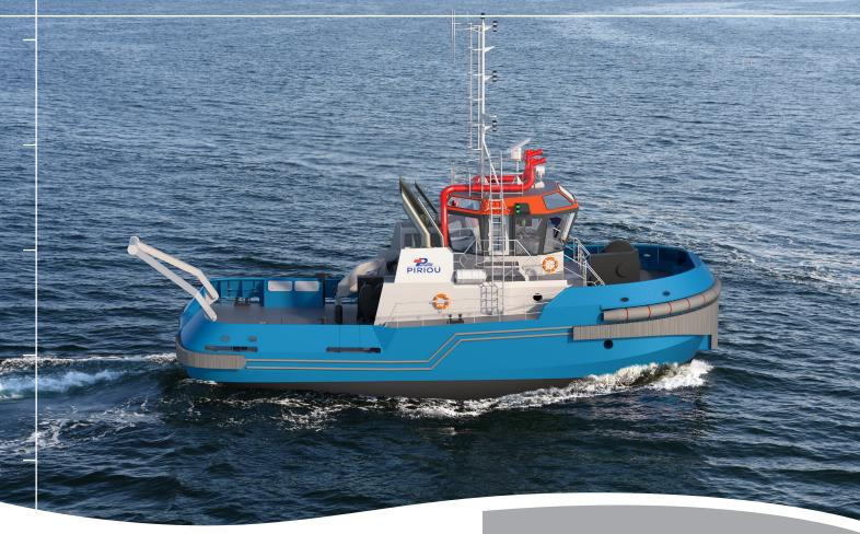
The OST 22 is a multi-purpose tug designed for pushpull towing and port assistance, as well as coastal towing operations. With a hull length of 22 meters and a width of only 8.75 meters, it has a bollard pull capacity of up to 35 tons.
